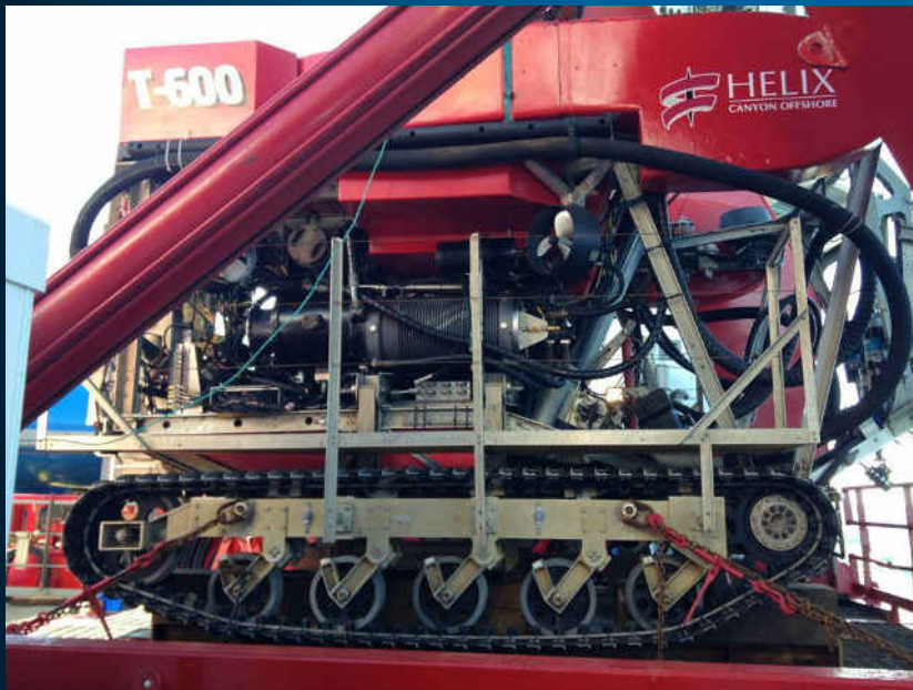
Remote Operated Vehicle (ROV) - 4000 m depth capability
